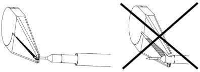
Spring loaded probe tips offer a method of probing signals that is less susceptible to vibration or movement than traditional rigid tips. Many users find it easier to use this type of tip. The spring loaded tips work when they are either partially or fully compressed and are protected against over compression damage.
